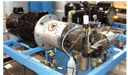
Maintenance-free sealing of proportioning pumps for polyol and isocyanate in high-pressure reaction casting machines
